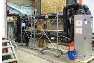
Fig. 2. HRV/ERV test rig
