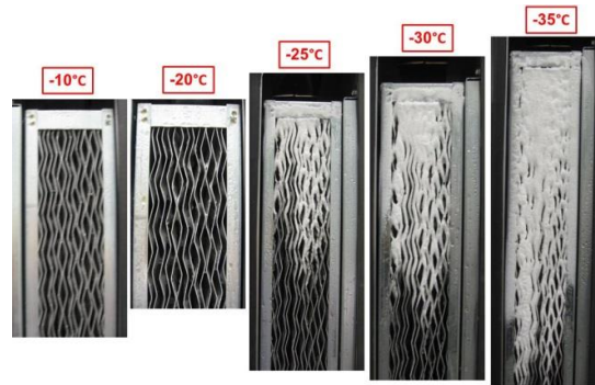
Fig. 7. Photos of the front top of the heat exchangers
